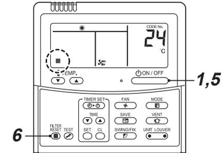
**1** Push the
