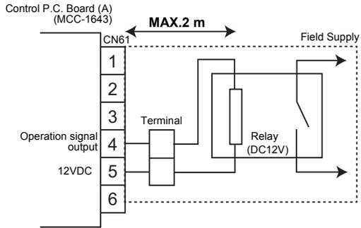
Contact is on during normal operation as factory default.
