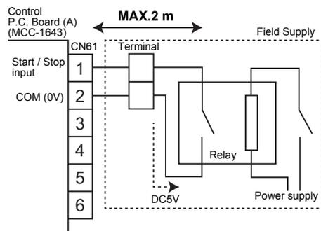
When the operation is linked by a signal from an external device or remotely controlled On and Off.
