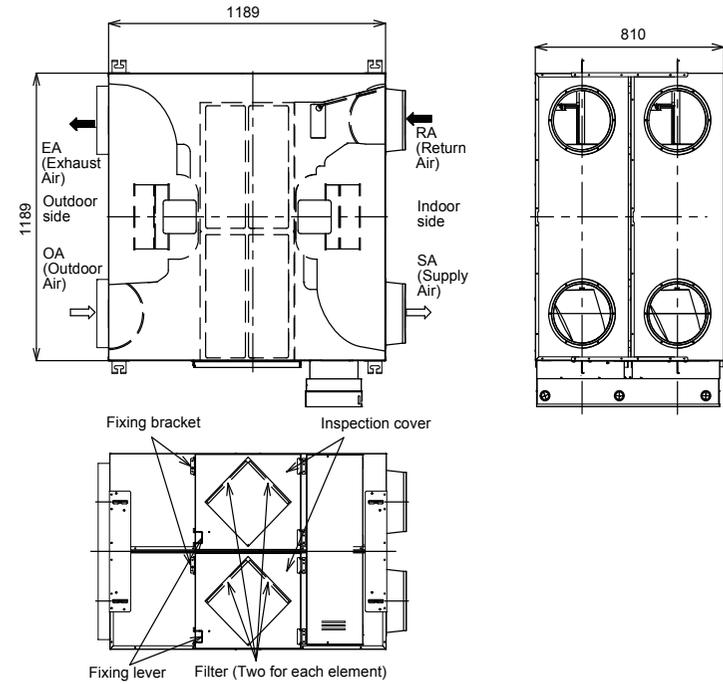
Applicable duct nominal diameter: indoor side Ø250
