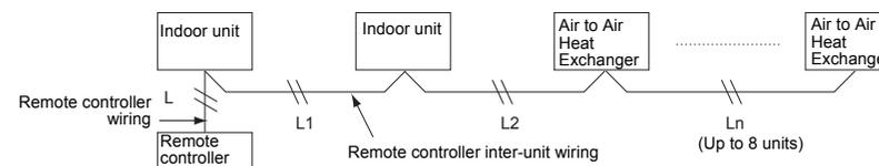
\* The total length of the remote controller inter-unit wiring is the same for both between the indoor units and between the Air to Air Heat Exchanger.
