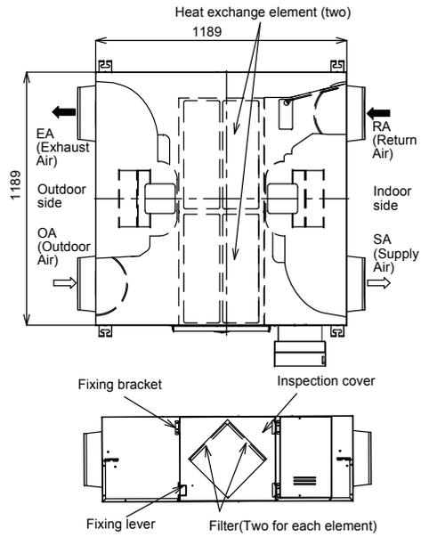
Applicable duct nominal diameter: indoor side Ø250
