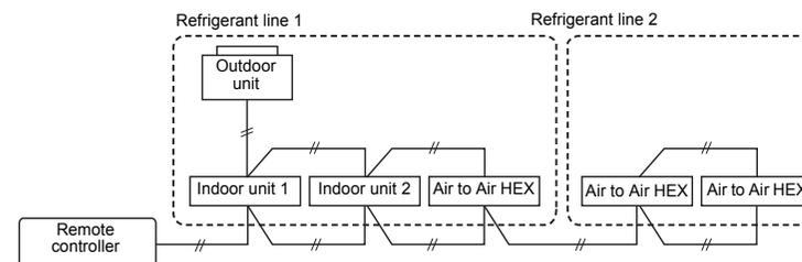
**Air to Air HEX can not be set the address even if the automatic address is set from outdoor unit in the system of Refrigerant line 1. Perform the address setting individually using remote controller. (Indoor unit 1,2 can be set the automatic address by the outdoor unit.)**
