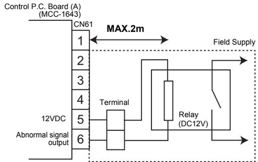
It is possible to monitor an abnormal signal from the Air to Air Heat Exchanger.
