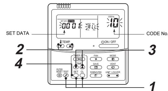
Pair the indoor unit to set and the remote controller one-to-one.
